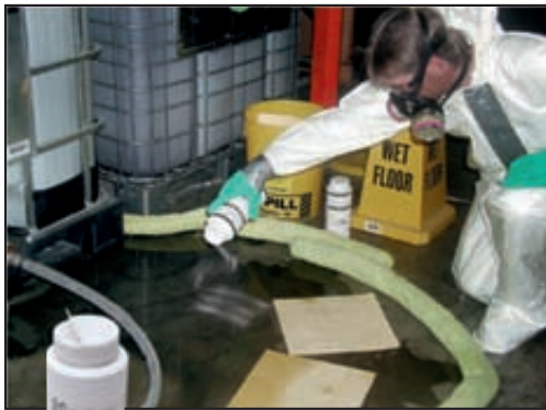
Dry formula is concentrated and thus has a greater neutralizing capacity versus liquid neutralizers.
